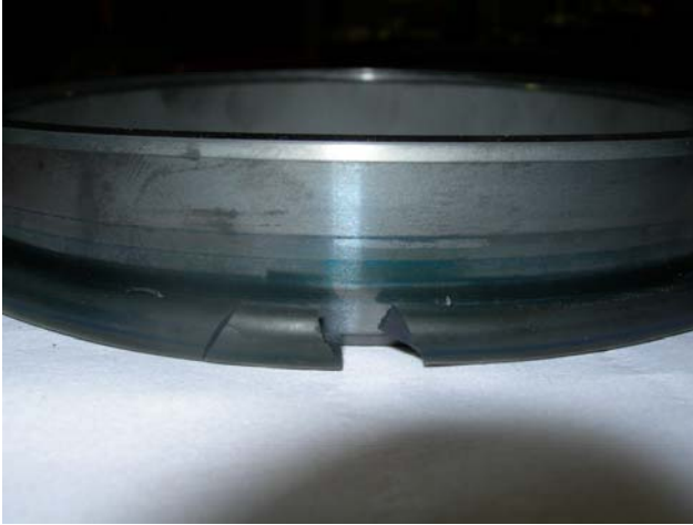
Fig.1 Inboard stationary seal ring O-ring showing section missing.
