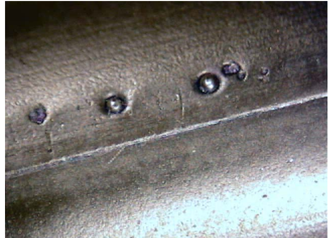
Fig.4 Inboard stationary seal ring O-ring showing beads embedded in the softened surface (ID /product side).
