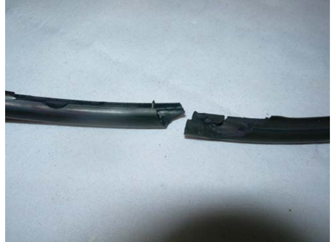
Fig.2 Inboard stationary seal ring O-ring showing nibbling and cracking
